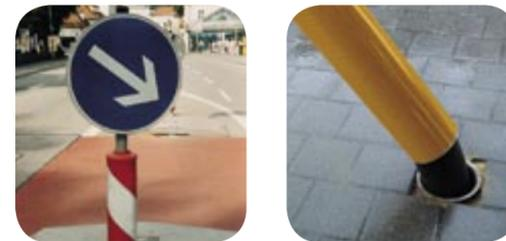
The Signal model is based on the Universal provided with a 250mm deep hole in the top. The hole is mounted with an Ø60mm galvanized steel pipe and on the top you find 3 x M8 screws which make it possible to attach a pipe of Ø46mm outer diameter. Alternatively the hole can have a Ø60mm pipe in full length. Furthermore it is possible to mount the Signal with an aluminum pipe provided with short light reflector in various colors.
